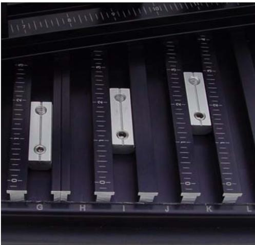
Photo #1 shows the T-slots and laser engraved reference system with T-nuts. The T-nuts have two threaded holes to allow the nut to remain locked in place while components are removed for other setups. Documentation of the fixture setup can be done with some simple notes and a digital photograph linked to the inspection program.
