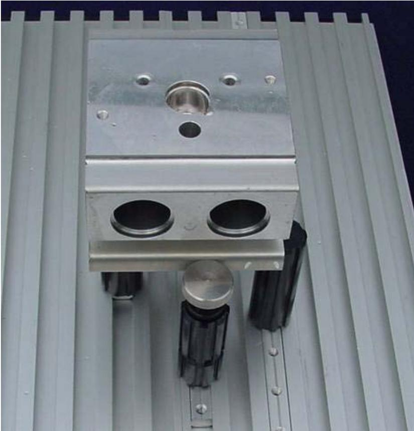
In summary, you will find that a variety of part shapes can be held with a simple six point fixture nest. In this basic example a very clean fixture with no overhead clamping is accomplished by sliding component a component in the t-slot and “pinching” the part against the fixture nest.
