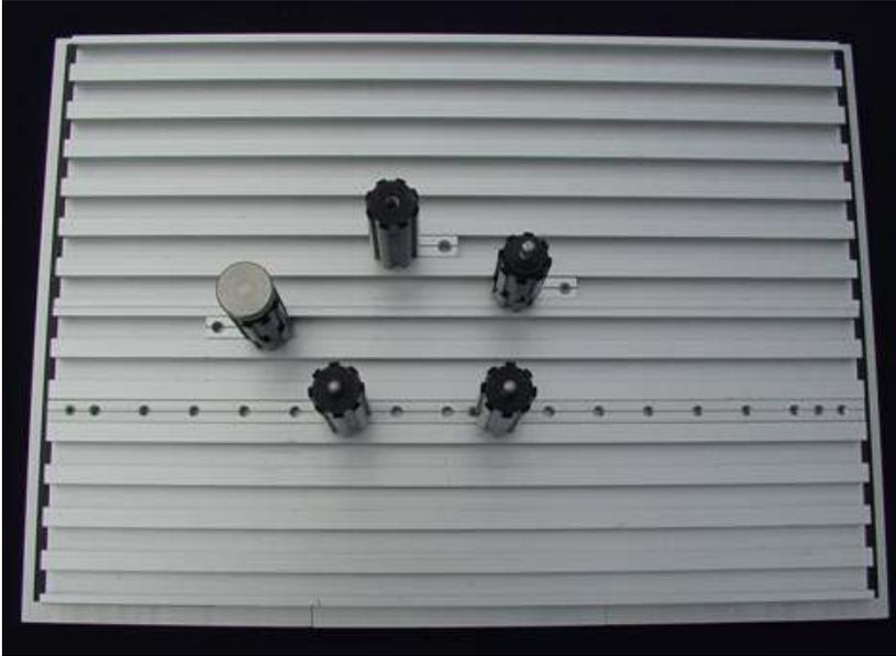
End view for tertiary locator. Note the set screw into the extra hole in the t-nut. This helps lock this locator in place securely. Also note the end locator doesn't make contact with the A datum.
