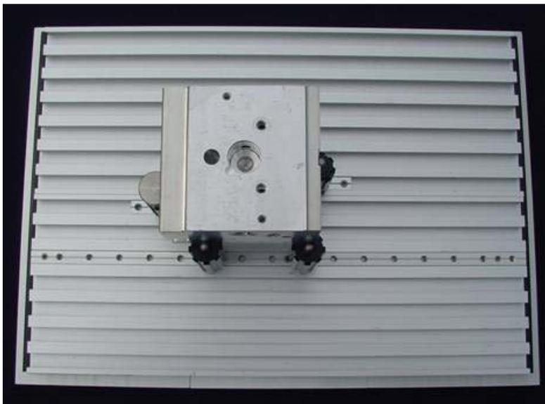
View of fixture without part. The bare standoff is the third A datum locator. Remember that the end-stop (tertiary locator) should not make contact with the A datum, it is an end locator only.
